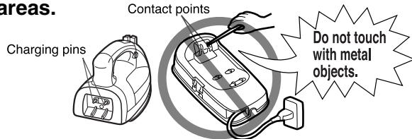
Touching the contact points with any pins or wires can cause short-circuiting, electric shock and fire.
